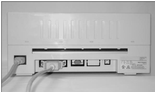
Make sure that the printer and the computer are switched off and connect the data cable between the printer and the computer, in this example a 36-pin centronics parallel cable.
