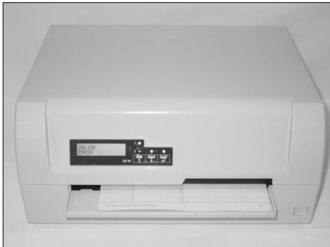
Place the passbook on the right-hand side of the document support with the page to be printed facing up. The passbook must be entered into the opening of the chute. Once in the chute the printer mechanism will take the book. At this point you may release the book, as the printer will align it against its right stop position and load it into the printer.
