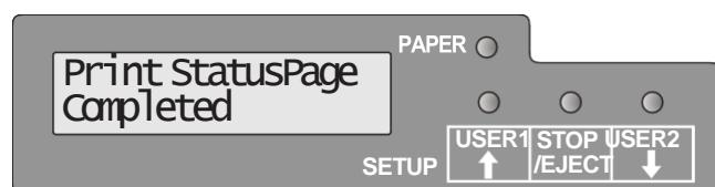
When the test printout is aborted or completed, LCD will display **Print StatusPage Completed**.
