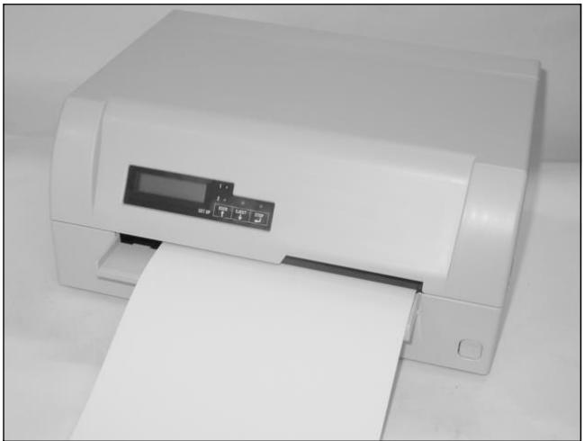
Insert the document in such a way that the right paper edge is positioned inside the area between the left side of the symbol and the right edge of the document support, so that the document alignment can grasp it securely. This is especially important for documents that are narrower than a DIN A4 sheet.
