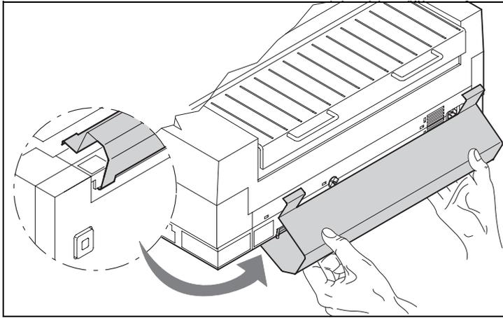
Hook the paper guiding bracket at the bottom of the printer as shown in the figure and then raise it until it clicks into place by exerting gentle pressure.
