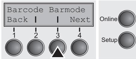
Allows printing of normal characters on the left and right of the barcode.
