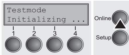
Enter advanced menu mode by pressing the **Online** key while switching on the printer.
