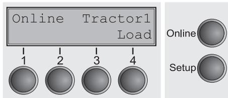
The active paper source appears in the display. By default, this is the paper path with the front tractor.
