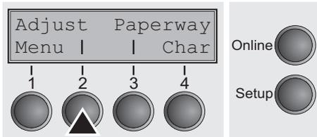
If the tear position of the paper is not aligned with the tear edge of the printer, you can adjust it. Inserted paper needs to be torn off if necessary and retracted to park position.
