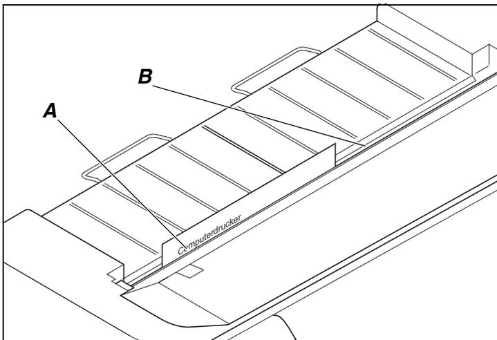
The paper is fed to the position where the bottom edge of the first printing line **A** is aligned with the tear edge **B** of the printer. The factory setting for the first printing position (TOF) is 12/72" (4,23 mm/1/6 inch). This is equivalent to the second line from the top.
