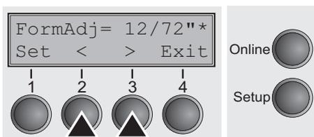
Press the **< (2)** or **> (3)** key to move the first printing line to the desired position. You can set values from 0 to 220/72" for fanfold paper.
