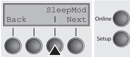
If the parameter **Sleepmod** is activated, the printer switches to energy-saving mode after 10 minutes of inactivity (<20 W).
