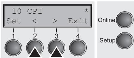
If you pressed the **Font** (2) key, use the < (2) or > (3) key to select the desired font. Confirm the selection by pressing the **Set** (1) key.
