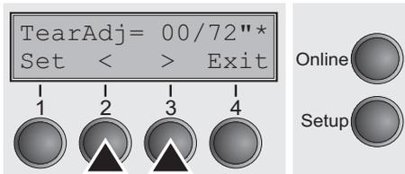
Press the < (2) or > (3) key to move the perforation to the desired position. Confirm the input by pressing the **Set** (1) key. Confirm the input again by pressing the **Setup** key. The printer is reset to the initial status.
