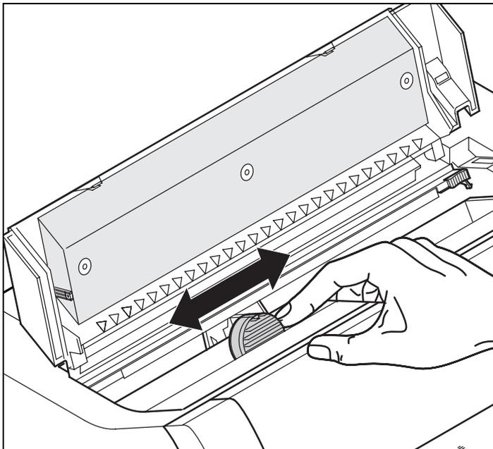
Move the print head carriage back and forth several times. If the ribbon is correctly seated, there must be no perceptible resistance.
