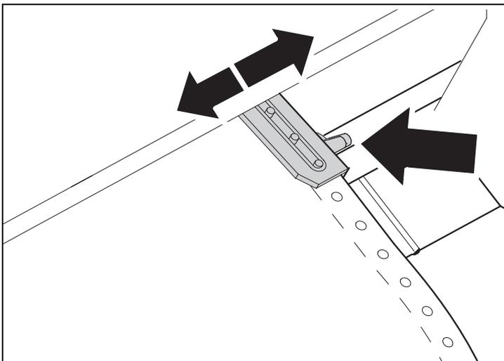
Open the coloured latch lever of the right-hand tractor and align it to the paper width.
