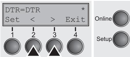
**DTR=DTR:** DTR signal is assigned to DTR line.
