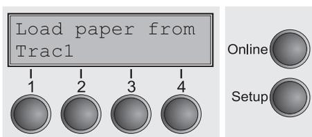
The paper is automatically loaded when the printer is in online mode and receives data from the computer.
