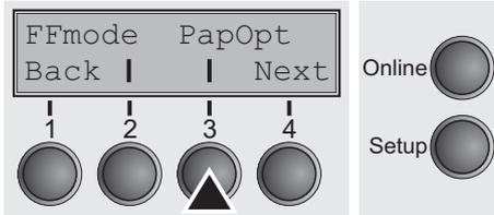
For setting the optional automatic sheet feeders (ASFs) and optional tractors; see [Paperway](#) (page 5). Also regulates the activation of ASFs and/or optional tractors.
