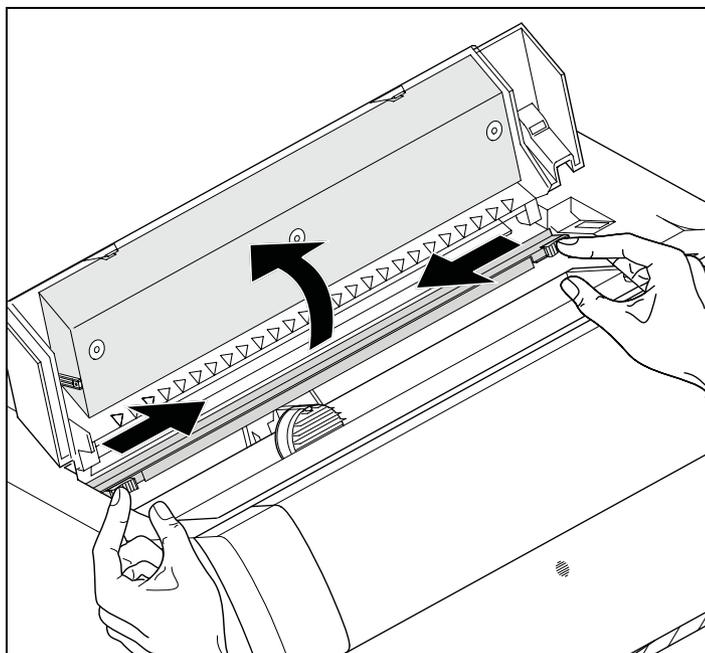
Move the coloured friction tabs to the left and right (direction of the arrows) as shown in the figure and raise the friction mechanism.
