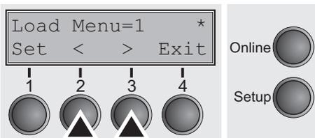
Confirm the setting by pressing the **Set** key (1). Press the **Next** key (4) to access the next group of parameters.
