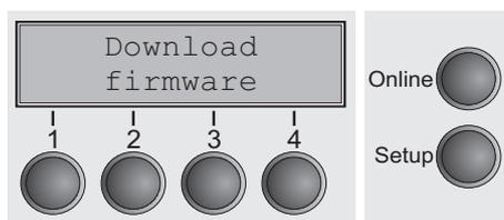
A progress indicator (bar) and DOWNLOAD FIRMWARE appears on the display during the download; alternatively, an error message is displayed:
