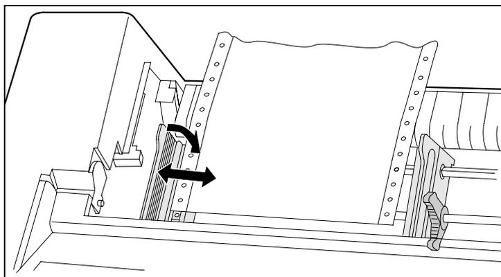
Release the coloured latch lever of the left-hand tractor and align the tractor in such a way that the first printing position on the paper matches the **X** mark on the printer housing.
