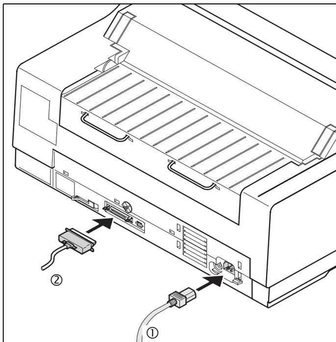
Connect the power cable ① to the power inlet of the printer. Connect the power cable plug to a mains socket.
