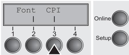
Use the < (2) or > (3) key to set the desired character density. Confirm the selection by pressing the **Set** (1) key.
