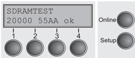
After switching on, the printer passes through a memory test during the initialization phase. In the display appears temporary the message "SDRAMTEST XXXXX XX ok".
