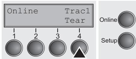
Make sure that the printer is in online mode. If necessary, press the **Online** key.
