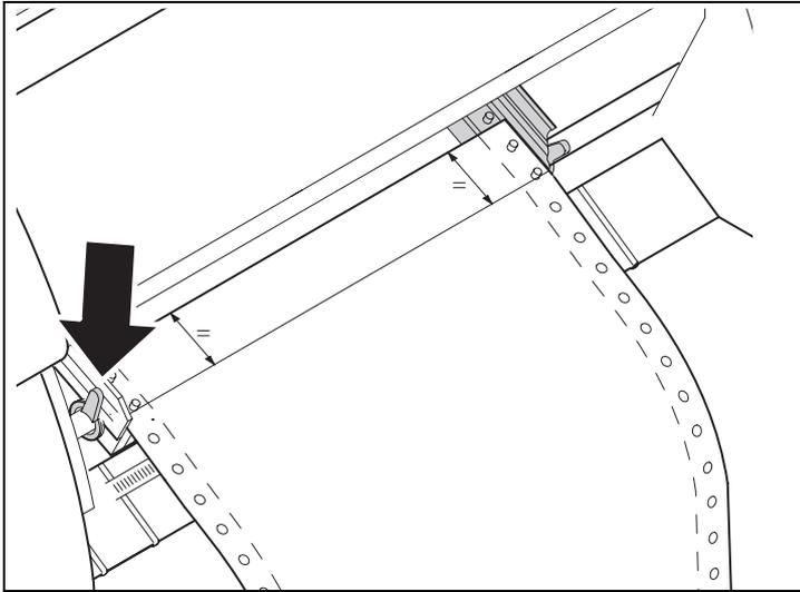
Release the coloured latch lever of the left-hand tractor and align the tractor so that the first printing position on the paper matches the **X** mark on the printer housing.
