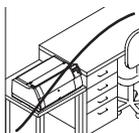
It is recommended to install the printer in a place which is acoustically isolated from the workplace because of the noise it may produce.
