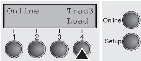
Press the **Online** key to select the printer. When the printer receives data from the computer, the fanfold paper will be loaded automatically.
