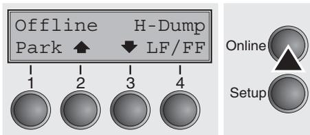
Put the printer into **Online H-Dump** mode by pressing the key **Online**. The printer is now ready to receive data from the computer and to print it out in hexadecimal format. The printed data can now be analyzed and evaluated.
