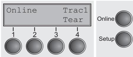
After switching on, the printer is automatically set to online mode. Only in this mode can it receive data from the computer.
