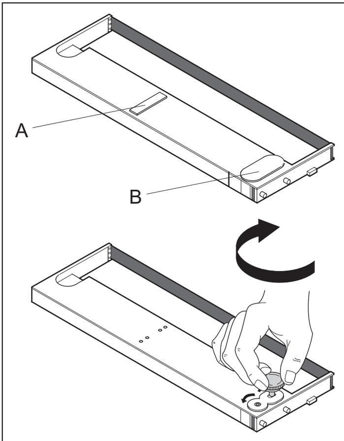
Remove the coloured protections **A** and **B**.
