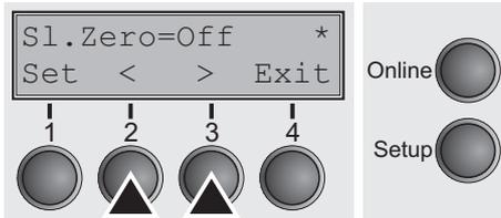
Confirm the setting by pressing the **Set** key (1). Press the **Next** key (4) to access the next group of parameters.
