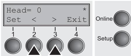
Use the **< (2)** or **> (3)** key to set the range within which the automatic gap adjustment is to be corrected. You can select values in the range from -10 to +10.
