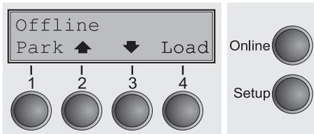
Only in this mode is it possible to perform step, line, or form feeds from the control panel, see [Paper transport \(page 42\)](#); however, data cannot be received.
