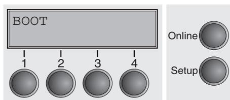
The printer is ready for the download when **BOOT** appears on its display.
