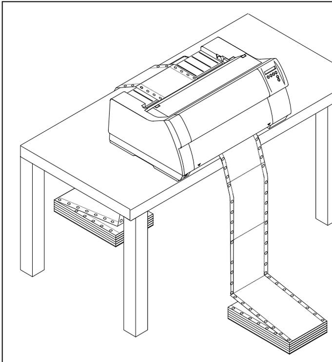
Place the printer on a solid, flat, surface, ensuring that the printer is positioned in such a way that it can not topple, and that there is easy access to the control panel and paper input devices. Also ensure that there is sufficient space for the printed output.
