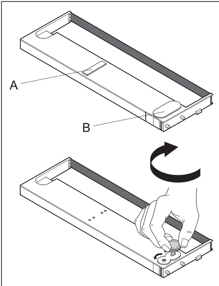
Remove the coloured protections **A** and **B**.
