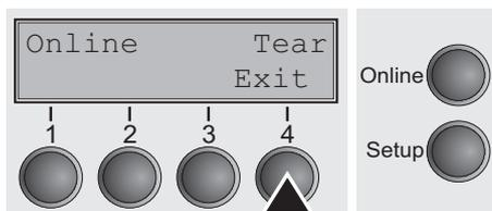
After having torn off the paper, press the **Exit** (4) key. The printer returns the paper to the first printing position.
