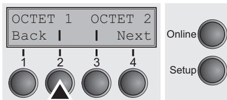
This menu level offers the possibility to set the IP address, which is divided into four digit groups (octet 1 to 4). You can activate octet 3 and 4 by pressing the **Next** (2) key.
